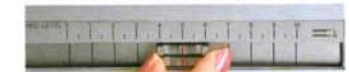
Sliding record level controls run parallel to the LED meters, making it simple to set proper record levels.
